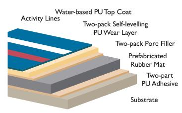
The substrate is usually high density macadam, concrete or a wooden base which is of suitable specification and construction for the expected loads and activities.
