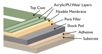
The cross section shows the key components in the **Sports-Cote<sup>TM</sup> Pro Elite** surface system.
